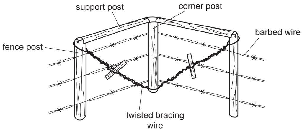
What does the twisted bracing wire help to support?
